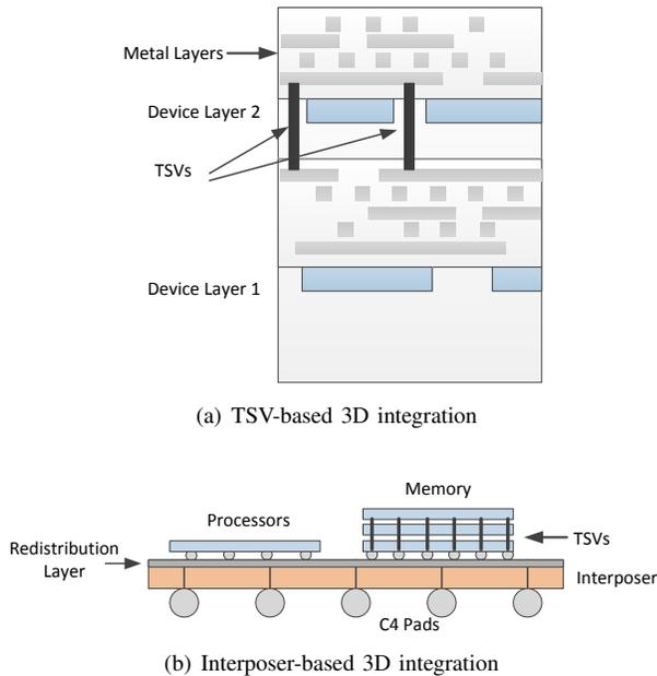
Fig. 1. A conceptual view of parallel 3D integration.
