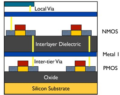
Fig. 2. A conceptual sketch of sequential/monolithic 3D integration.
