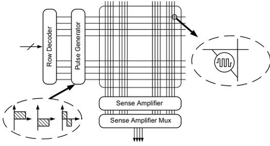
Figure 5: Structure of memristor based memory.
