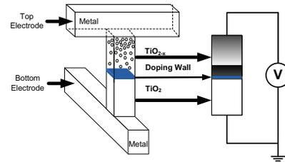
Figure 1: Structure of memristor cell.
