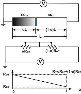
Figure 2: Circuit model of memristor [2].
