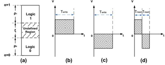
Figure 4: Write/Read operation of memristor based memory cell.
