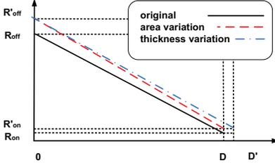
Figure 7: Resistance under the area and thickness variation.
