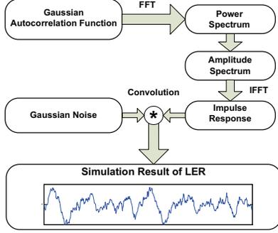
Figure 10: Process to simulate LER.
