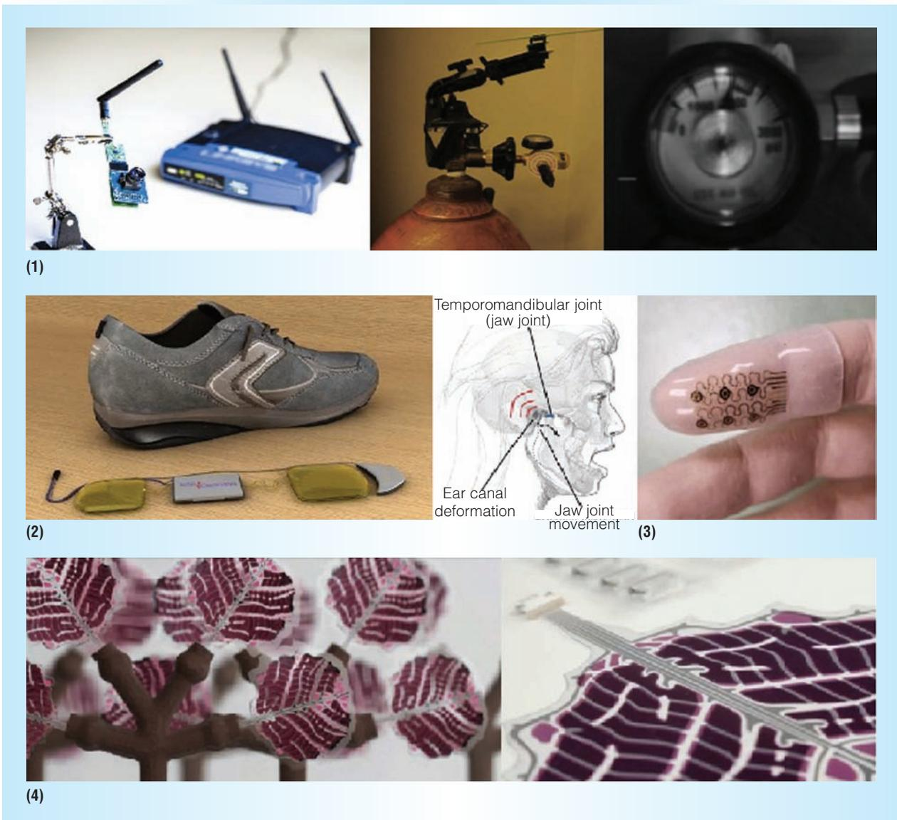
Figure A. A sampling of energy-harvesting Internet of Things devices. (1) A Wi-Fi-powered camera, with demonstration system mounted on an industrial gas cylinder, monitoring a pressure gauge.<sup>7,8</sup> (2) In-shoe piezoelectric devices<sup>9</sup> and a piezoelectric ear canal motion energy harvester.<sup>10</sup> (3) Thermoelectric generator.<sup>11</sup> (4) Solar leaves.<sup>12</sup>
