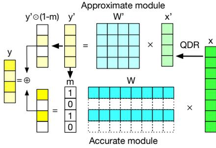
Fig. 3. Illustration of dual-module processing. The approximate module with quantized and dimension reduced (QDR) weights  $W'$  and inputs  $x'$  spends low-cost computations on intermediate results  $y'$  that are further used to generate the dynamic switching map  $m$ . With dynamic switching, the expensive computation and data access of executing the accurate module are saved. The final pre-activated vector  $y$  is a mixture of accurate and approximate results.
