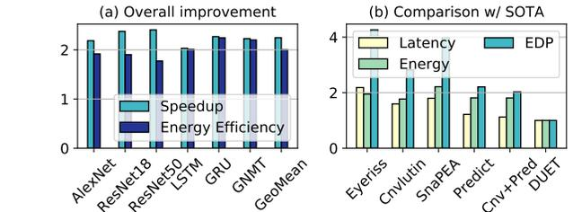
Fig. 11. (a) Overall performance speedup and energy efficiency; (b) Comparison with other accelerators.
